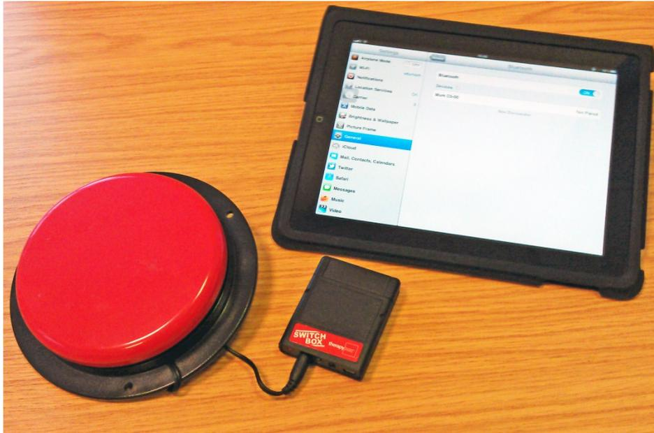
Figure 58: Using switch access with an iPad.
