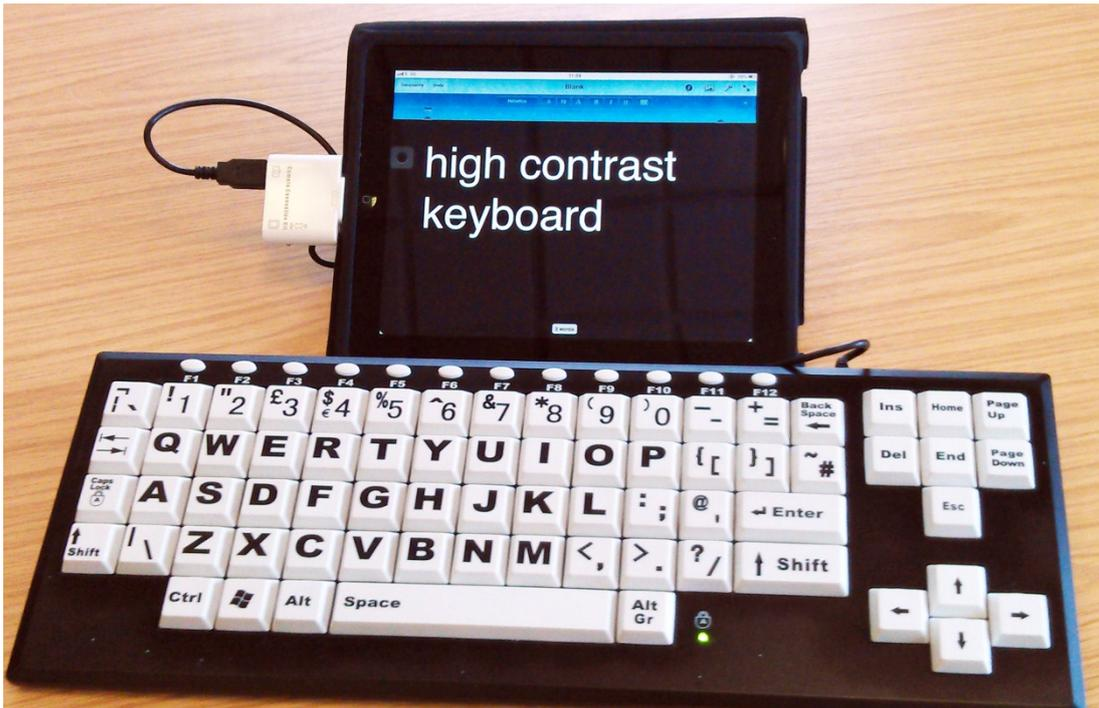
Figure 57: Example of high contrast keyboard connected to the the iPad via the USB Camera Connection kit.
