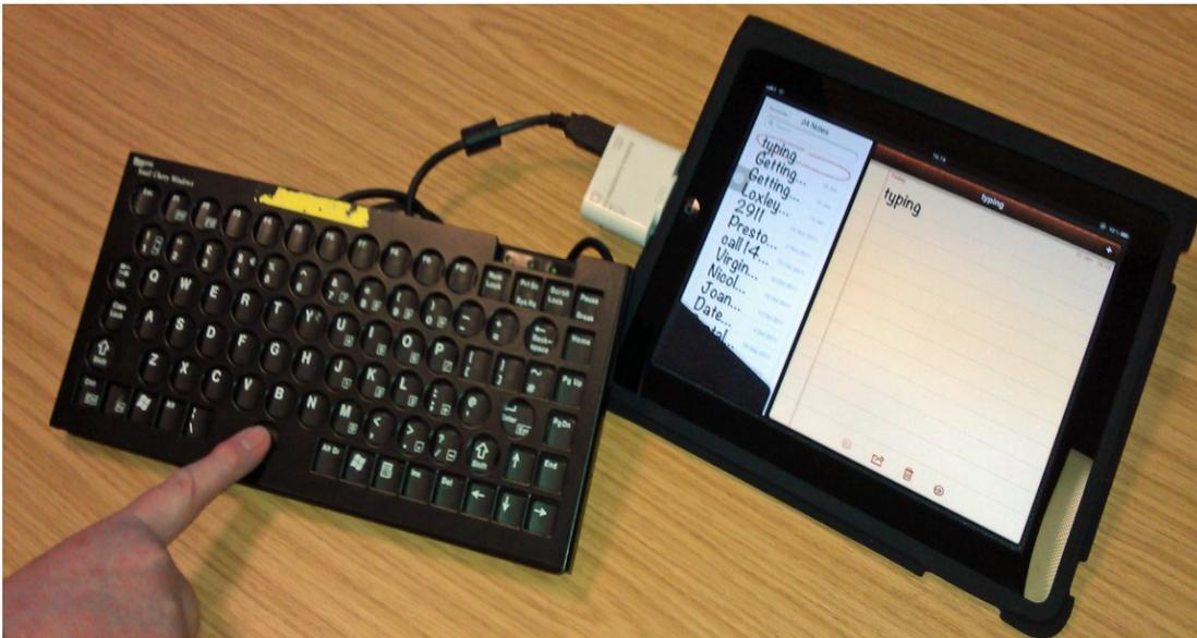
Figure 56: Example of a compact keyboard with keyguard using the USB Camera Connection Kit.
